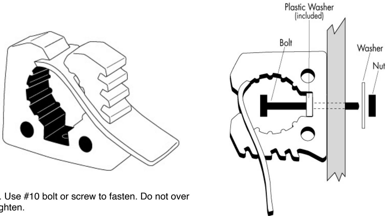
1. Use #10 bolt or screw to fasten. Do not over tighten.
